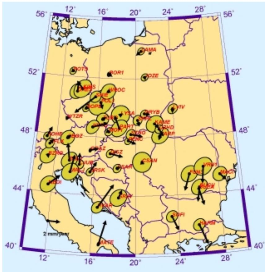
**Fig. 3** Estimated horizontal velocities and their  $2\sigma$  error ellipses of CEGRN sites observed more than 3 times and covering time span longer than 4 years.
