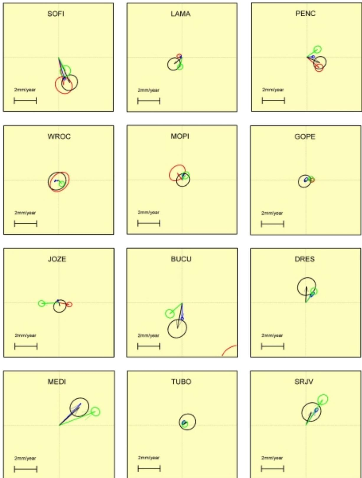
**Fig. 5** Comparison of velocities obtained from CEGRN epoch campaigns (black lines) with ITRF 2000 velocities reduced for APKIM 2000 (red lines), EPN velocities (blue lines) and velocities obtained from analysis of permanent stations in Central Europe (green lines).
