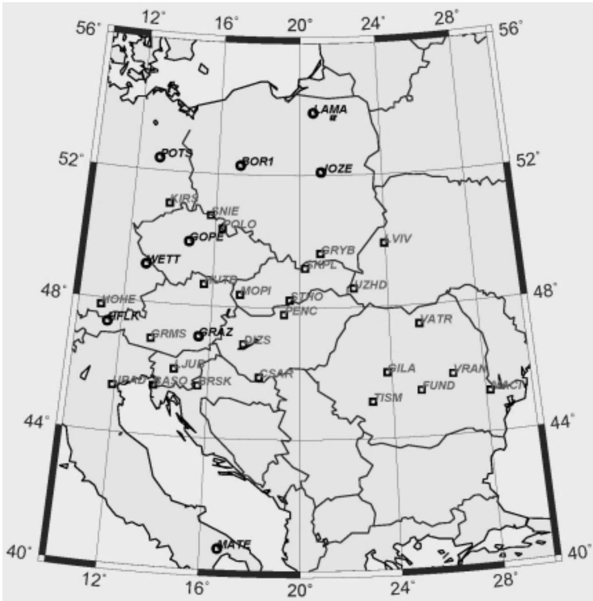
**Fig. 1** CEGRN constellation in the second observing campaign performed in 1995 (○ permanent stations, □ epoch stations).
